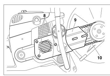
Unscrew the screws (8) and remove the crankcase housing cover (9).
