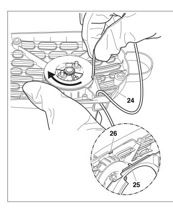
Guide the cable into the recess (24) on the cable drum and use the cable to turn the drum two turns in the direction shown by the arrow.
