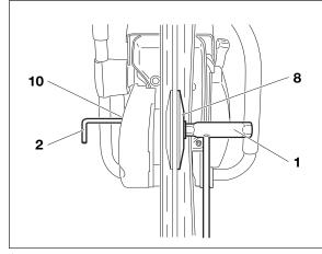
Place the spring washer (8) on the arbour and insert the screw (9) and tighten by hand.
