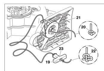
Thread in a new starter cable (dia 4.0 mm, length 1000 mm) as shown (don't forget the disc (19)) and knot both ends.
