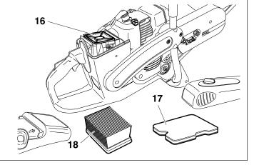
**CAUTION:** Turn off the engine before cleaning the air filter! Never clean out the air filter with compressed air! Do not clean the pre-filter and inner filter with fuel.
