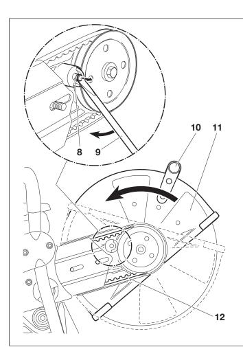
Use the combination tool (9) to lever out the stop pin (8) as shown in the illustration, until the protective hood (11) can be turned.
