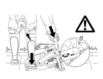
Grasp the tubular handle firmly with one hand and press the Power Cut against the ground.
